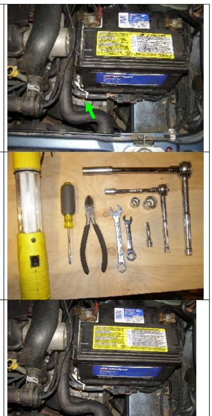
Remove the battery mounting plate 4x 10 mm
