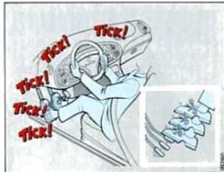
ABS braking - indication that the system is operation
