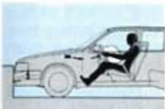
The sensor has registered the decrease in speed and sends a signal to a gas generator, via the control module, which inflates the airbag.
